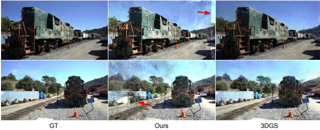
Figure 8. Failure case. On scenes with severe exposure variation of training views, our method struggles and produces clear boundary of different brightnesses and allocates many floaters. 3DGS on the other hand is less sensitive to photometric variation of GT. This explains our worse PSNR and FPS on Tanks&Temples in Tab. 2.
